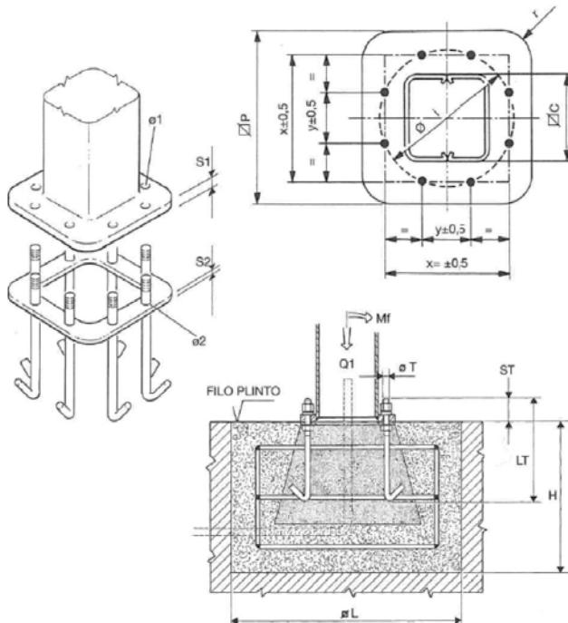
N.B.: The foundation frames with lug bolts, used in the column-mounted version for fixing the column itself to the foundation plinth is supplied on request.
