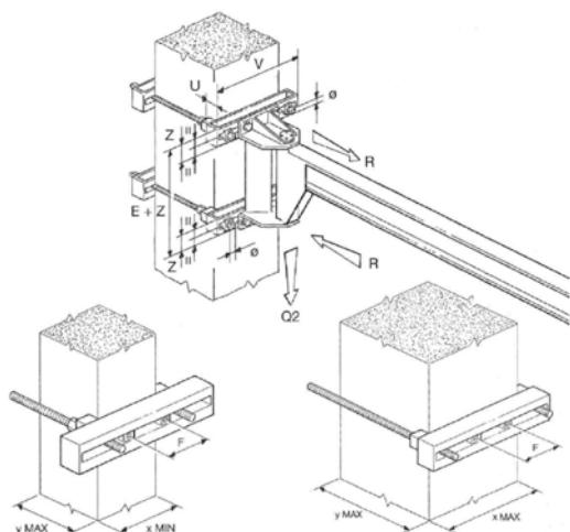
N.B.: The bracket and staybolts unit, used in the wall-mounted version for fixing the bracket to a pillar, is available on request.
