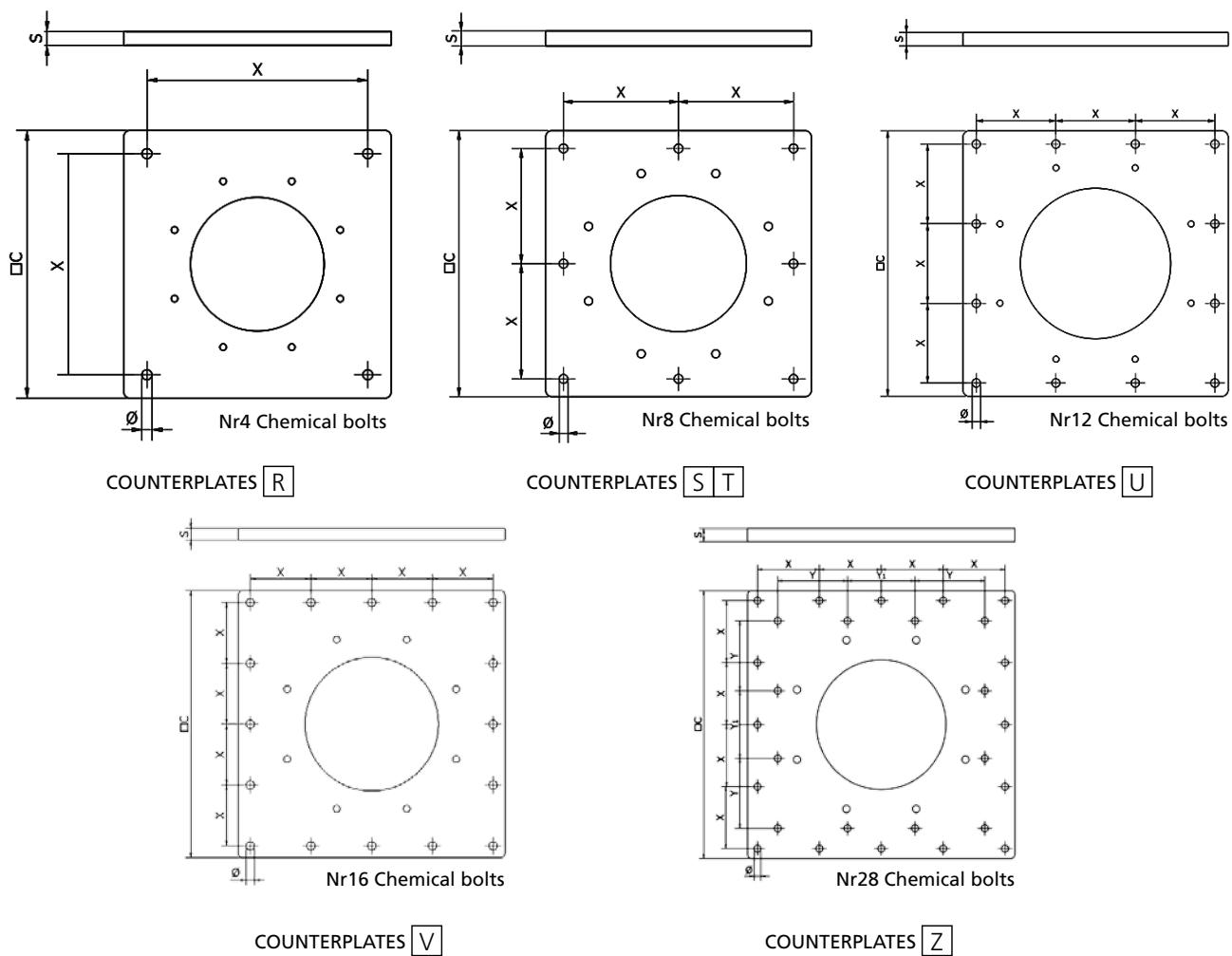
**The fixing of the column using chemical bolts, needs a scrupulous check of suitability in relation to the type of support flooring. The suitability checks are the responsibility of the user and must be carried out by expert, qualified technicians who will evaluate the feasibility and formally undertake the relative responsibilities.**
