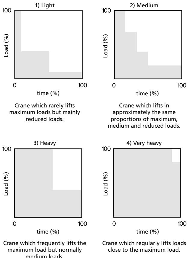
Check, on the basis of the stress level intended for the crane, that the limits of use, type of service and n° of cycles intended in 10 years of work are not in contrast with the following table.
