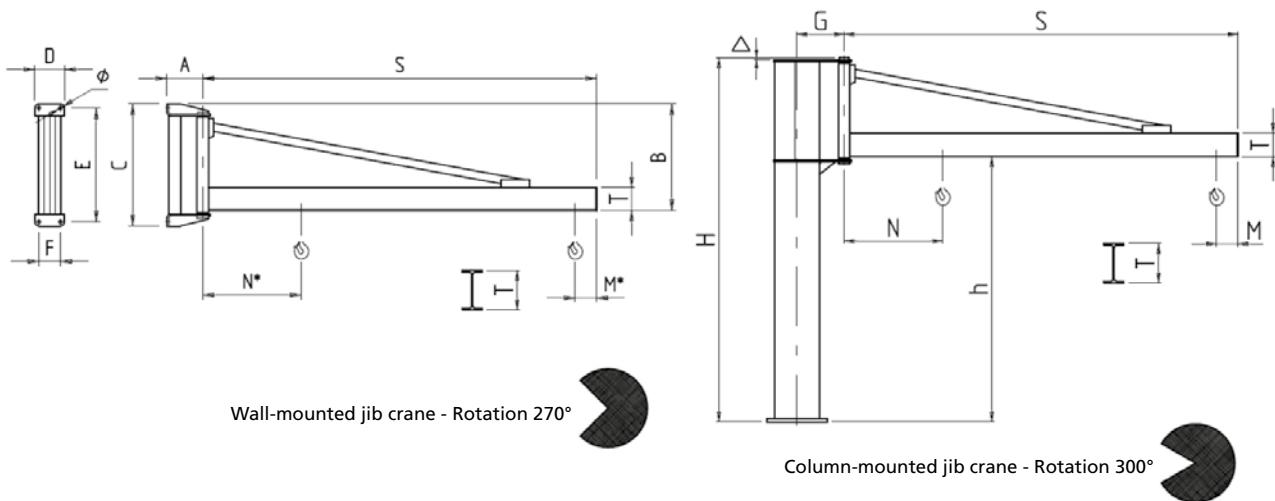
Heights M\* and N\* for wall-mounted jib cranes. See corresponding heights relative to column-mounted jib cranes.
